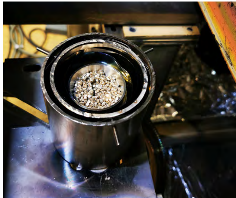
Evaporation crucible with lithium granules © Fraunhofer FEP
